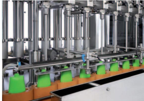
The linear filler has eight filling positions and is equipped with 1 l-metering cylinders.
