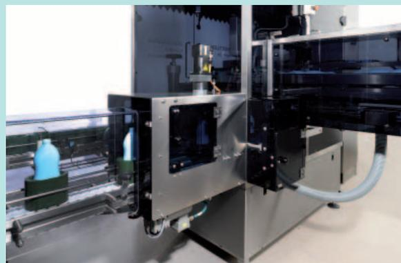
The empty containers that are supplied in bulk reach the pre-sorter of the Bottlemat via an elevator (left).
